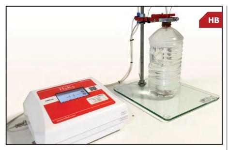
The H5K5.HB is an instrument designed to test the deformation of plastic bottles (Bulge test / Collapse test) by pressure difference in a easier, faster, efficient and standardized way.
